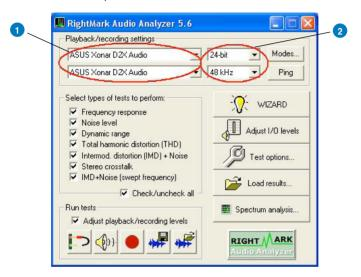
Click "Test options" button in RMAA and check "Analyze noise and distortion only in 20Hz-20KHz range" (audio in-band for human hearing) in the General tab.
