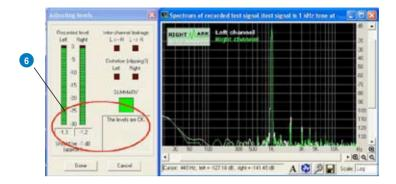
7. If the recording volume level is not high enough, please check and make the WAVE and Master Volume have been at the maximum level; Instead, if the recording volume level is too high, please lower the WAVE and Master volumes gradually until the level is ok.
